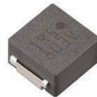
Outer Appearance of Liquialloy™ Inductor
